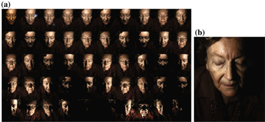
Fig. 3.18 a 50 input images for PTM: lights individually from 50 different directions e^i, i = 1 \dots 50 ; b interpolated image under new light e
