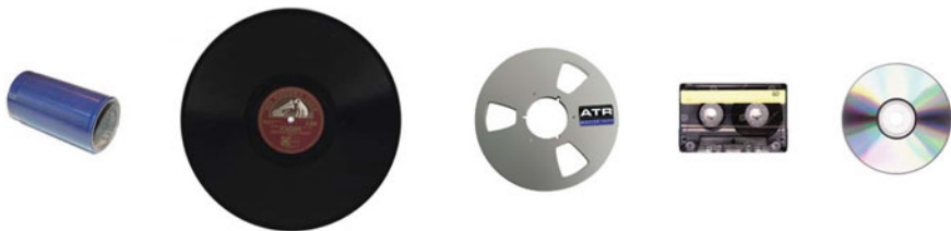
Fig. 1.3 Evolution of audio storage media. Left to right an Edison cylinder record, a flat vinyl record, a reel-to-reel magnetic tape, a cassette tape, and a CD
