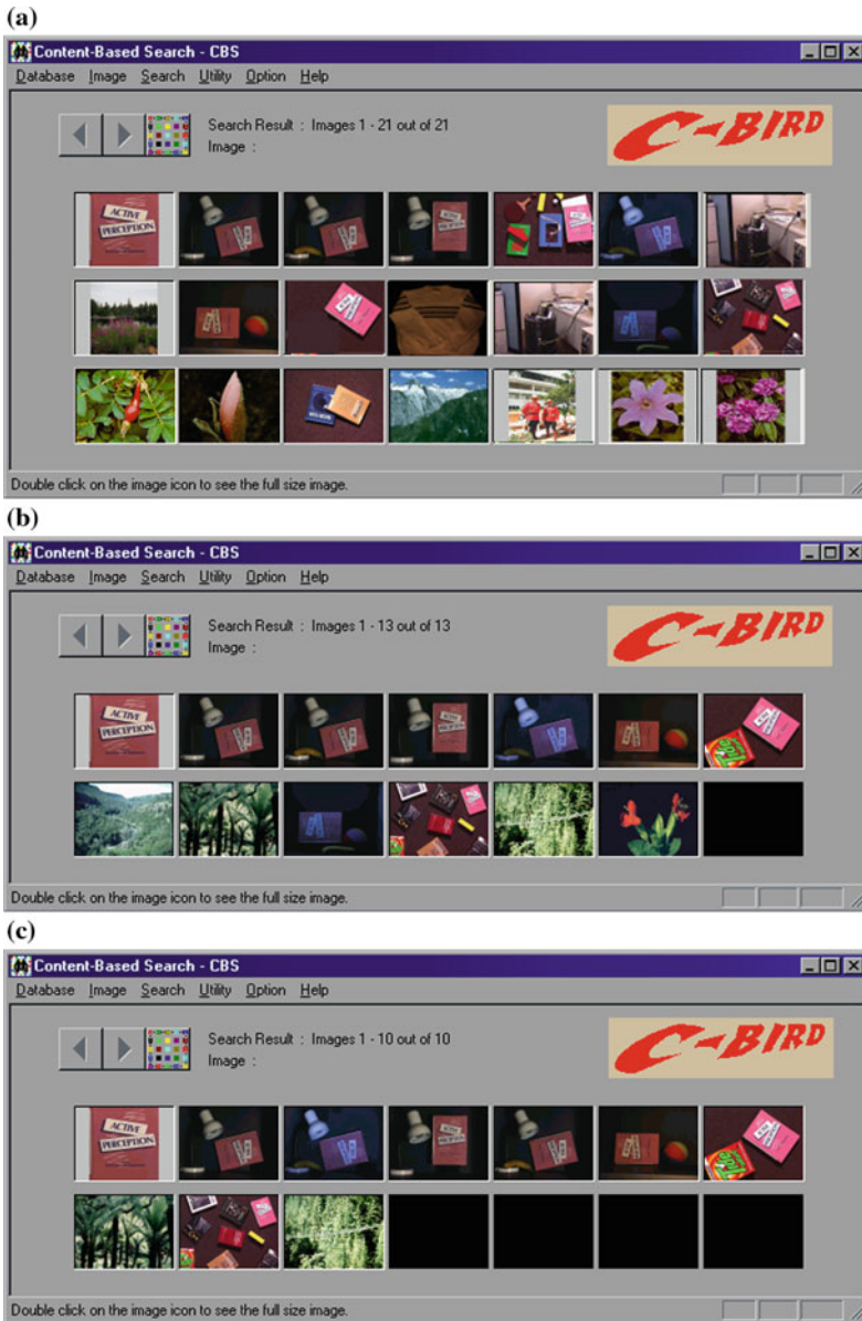
Fig. 20.9 Search result for the pink book model with illumination change support: a search results using pose estimation only; b search results using pose estimation and texture support; c search results using GHT shape verification. (Some thumbnail images are from the Corel gallery and are copyright Corel. All rights reserved)
