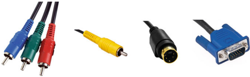
Fig. 5.7 Connectors for typical analog display interfaces. From left to right: Component video, Composite video, S-video, and VGA
