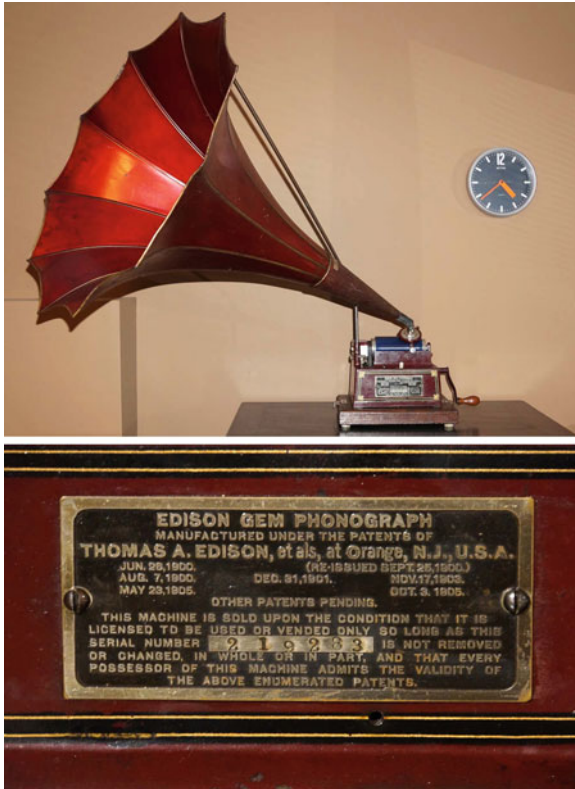
Fig. 1.2 An Edison phonograph, model GEM. Note the patent plate in the bottom picture, which suggests that the importance of patents had long been realized and also how serious Edison was in protecting his inventions. Despite the warnings in the plate, this particular phonograph was modified by the original owner, a good DIYer 100 years ago, to include a more powerful spring motor from an Edison Standard model and a large flower horn from the Tea Tray Company
